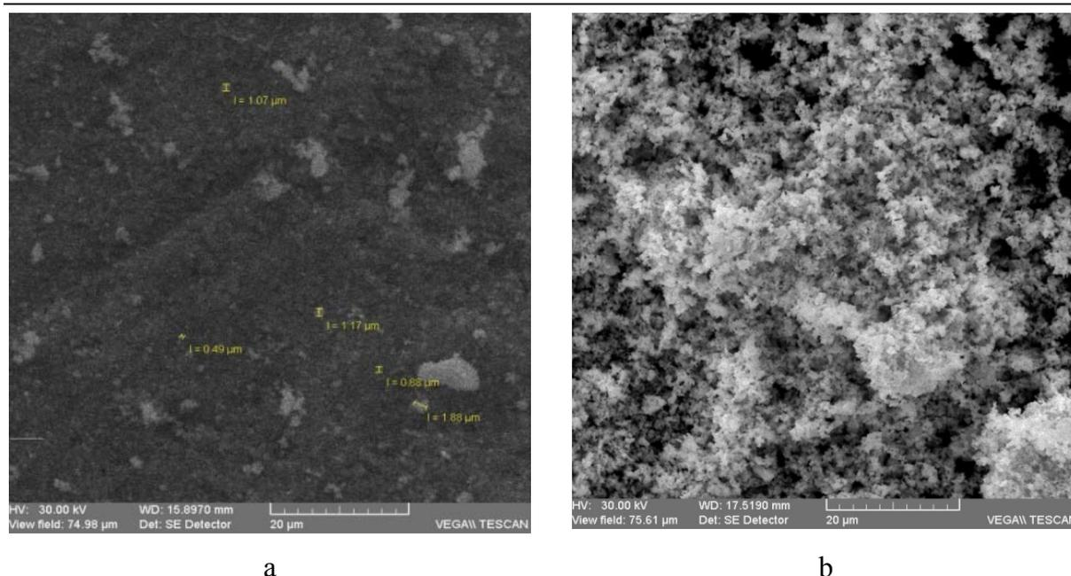
**Figure 4.** Scanning Electron Microscopy of  $\text{LaCoO}_3$  samples obtained by: a) chloride precursors annealed at  $800\text{ }^\circ\text{C}/4\text{h}$  and b) nitrate precursors annealed at  $950\text{ }^\circ\text{C}/4\text{h}$ .
