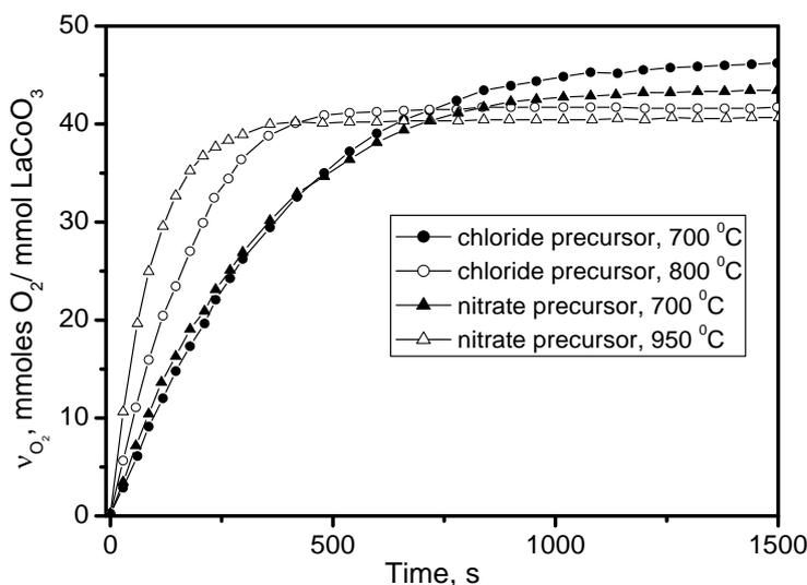
**Figure 6.** Variation of O<sub>2</sub> quantity with time in presence of lanthanum cobaltite as catalyst.
