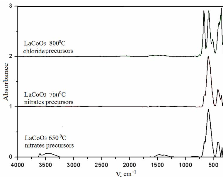
**Figure 5.** IR spectra of LaCoO<sub>3</sub> powders.
