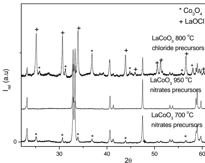
**Figure 1.** XRD powders obtained using chloride and nitrate precursors sintered at different temperature.
